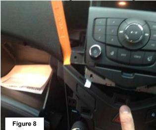
**6.** Remove the radio control panel by grasping and pulling towards the rear of the vehicle, and remove the 1 connector. This connector has a small blue clip which needs to be disengaged before it can be unlocked. Refer figure 9 and 10.
