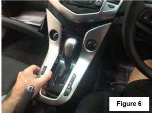
**4.** Remove the 8 x 9/32" bolts at the below points. After the bolts have been removed remove the storage pocket. Refer figure 7
