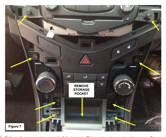
**5.** Pull out climate control panel at the following point. This panel can be very hard to remove. Be patient and the clip will remove. Repeat on the other side. The panel can be covered with a towel or suitable protective material and allowed to hang to the side. Refer figure 8.
